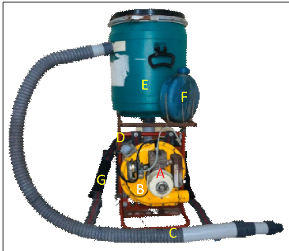
Fig. 6 : Modified knapsack cotton picker. A - Engine, B - Aspirator, C - Sucking assembly, D - Mounting frame, E - Collector with filter, F - Fuel tank, G - Shoulder straps.
