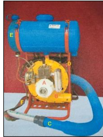
Fig. 1 : View of existing knapsack cotton picker (Kathiria, 2011). A - Engine, B - Aspirator, C - Sucking assembly, D - Mounting frame, E - Fuel tank, F - Shoulder straps.
